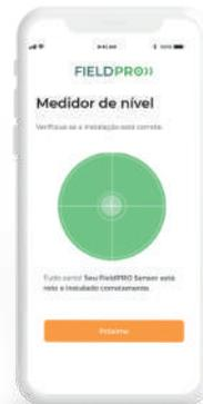
The bubble level that moves on your smartphone screen must be positioned right in the center. The bubble will turn green when it is in the center, indicating that your Sensor is correctly installed.
