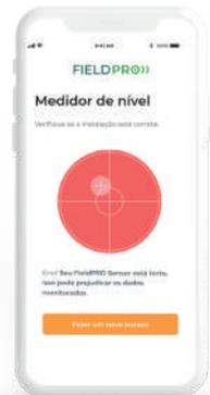
If the bubble is not in the center, it means your Sensor is tilted.
