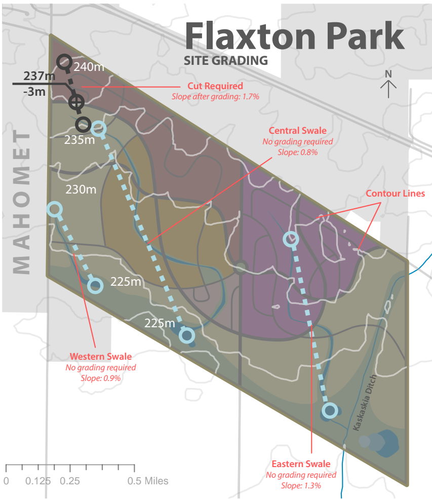
FIGURE 10: Site Grading for Flaxton Park By using the site’s natural slope, Flaxton Park minimizes cut-and-fill, preserving the natural permeability of the soil.
