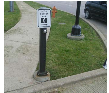
Pushbuttons within 10 Feet of the Curb
