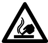
This symbol indicates the presence of parts with high temperatures.
