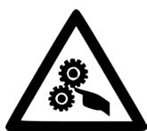
This symbol indicates the presence of moving parts inside the machine.
