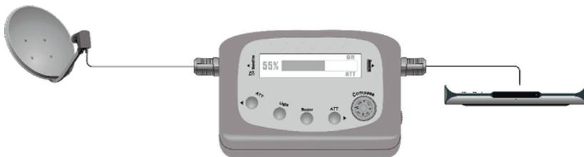
1. Connect the coaxial cable from LNB (satellite dish) to the LNB connection of the SAT FINDER (1).
