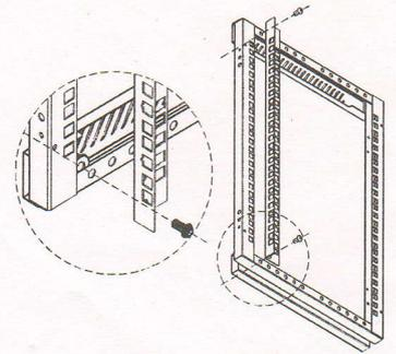
【3】 Fix 19" mounting rails to the first holes of top & bottom of side frames by 4sets of M5 screws.
