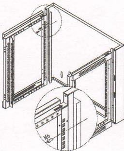
【4】 Install side frames to the grooves of back frame by 4pcs of M6\*12 screws (6pcs if more than 18U) as shown by the arrow in the picture, note 19" mounting rails are in the front side.
