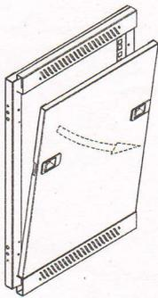
【1】 Remove ⑦ from ②, put them separate for the preparation of the frame assembly.
