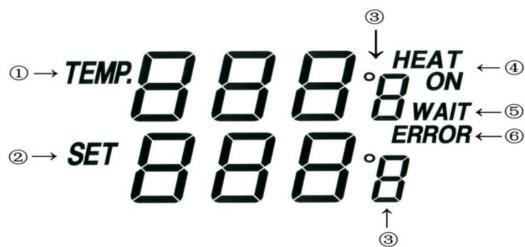
1. TEMP: Temperatura real do ferro de soldar
