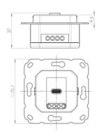
Connection: screw terminals up to 2,5 mm<sup>2</sup> (rigid)
