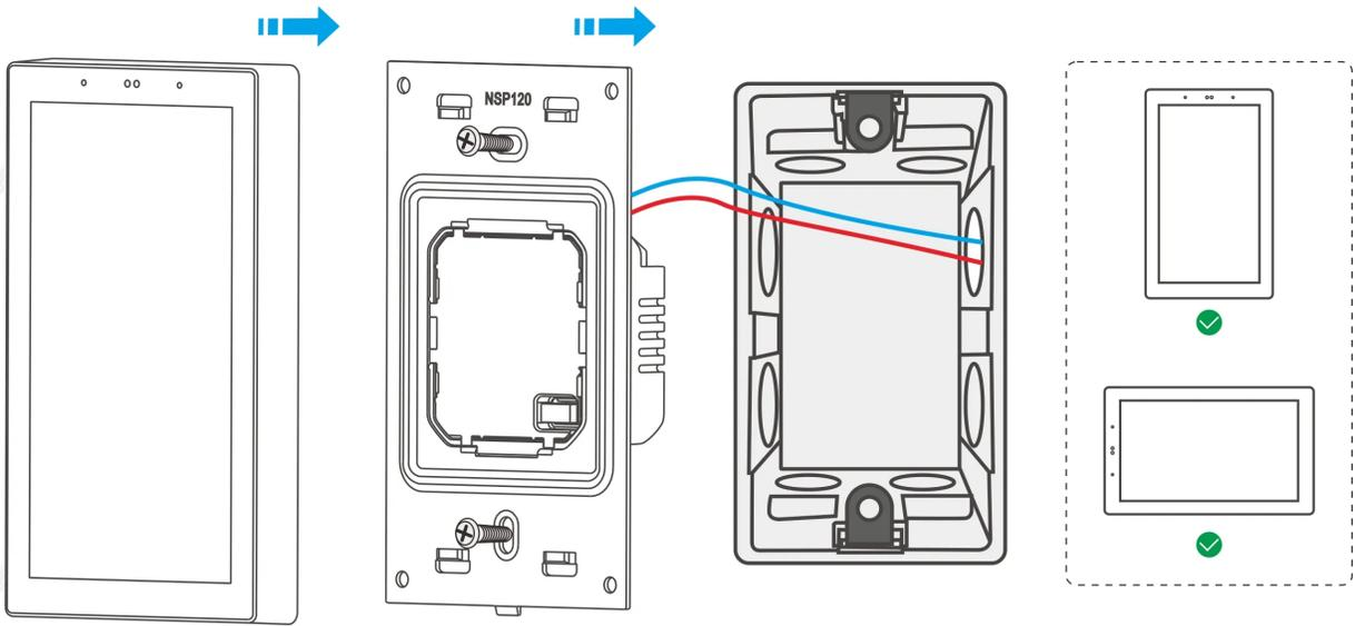
\*The product should be installed in the concrete wall or other non-combustible location.
