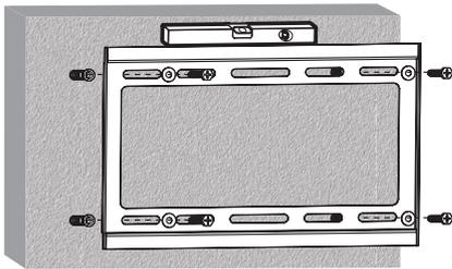
Install the wall plate to the solid wall
