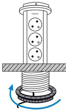
Remove the detachable locking ring from the socket, and put the socket into the hole.
