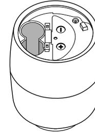
\*Do NOT use rechargeable batteries or 1.2V AA batteries.
