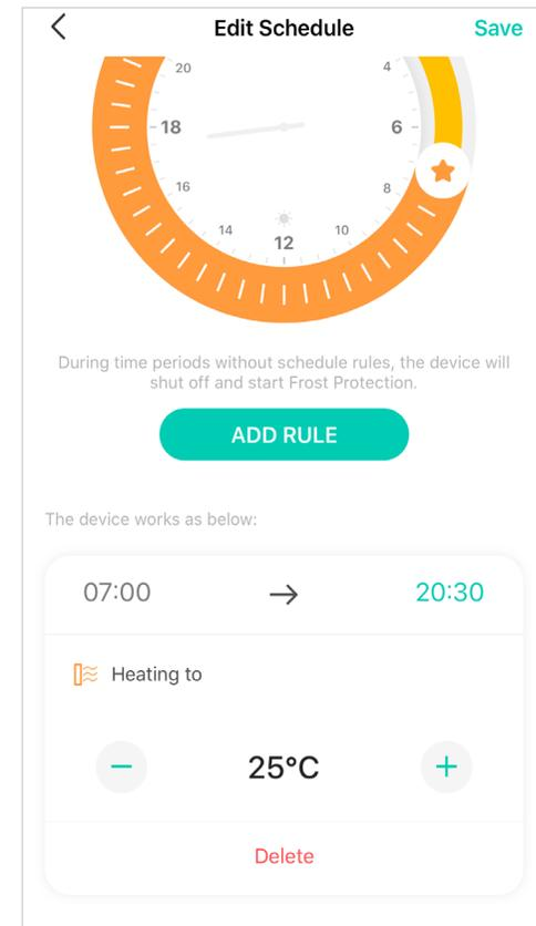
7. Tap **Save** and your smart thermostatic radiator valve will heat to 25°C from 7:00 am to 20:30 pm on weekdays.
