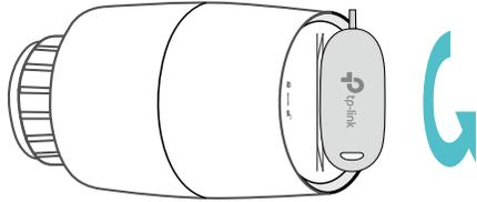
4. Open the battery cover and insert two AA LR6 Alkaline batteries. Make sure the positive and negative terminals face the correct direction.
