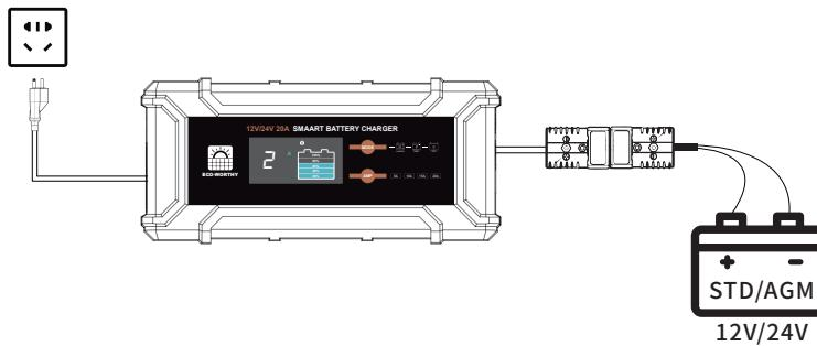
9. Lithium Battery Activation Mode: After selecting the LFP mode, connect the lithium battery that needs activation to the charger to automatically begin the activation process, which defaults to the 12V activation mode. And press and hold for 3 seconds in the LFP mode to switch to the 24V activation mode.
