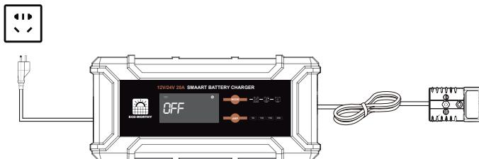
2. LFP Mode: After selecting the charging mode and current for lithium iron phosphate (LFP) batteries, simply connect the charger to the battery to start charging (the battery voltage is automatically recognized). Once the battery is connected, it is not possible to switch the battery type, but it can change the charging current (12V: 5/10/15/20A; 24V: 5/10A).
