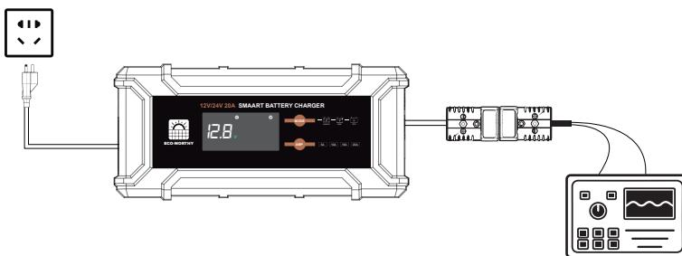
6. AGM Recovery Mode: In AGM mode, press and hold for 3 seconds to enter the AGM recovery mode (only applicable to 12V lead-acid batteries). This mode is used to repair old, idle, damaged, stratified, or sulfated batteries by applying pulse charging at 15V. Once the battery is connected, it is not possible to exit the recovery mode, and the pulse charging will be turned off after two hours (charging current can be switched during this period).
