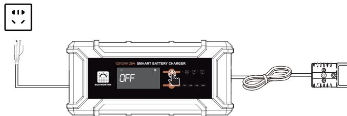
2. Connect the battery to one of the included Anderson cables (red end for positive, black end for negative).
