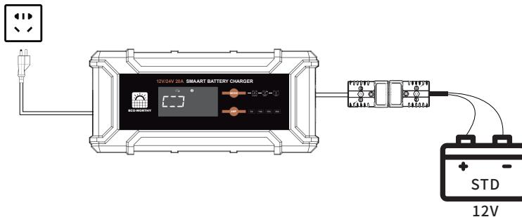
8. Low-Temperature Charging Mode: Select the low-temperature charging mode and connect the charger to the battery. The charger will use a small current (2A for a continuous 5 minutes) to charge it, then switch to the normal charging current. This mode is only applicable to 12V/24V lead-acid batteries (STD, AGM).
