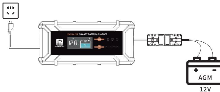
4. STD Mode: After selecting the STD battery charging mode and charging current, you can start charging by connecting the charger to the battery (the battery voltage is automatically recognized). Once the battery is connected, it is not possible to switch the battery type, but it is possible to change the charging current (12V: 5/10/15/20A; 24V: 5/10A).
