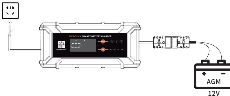
7. STD Recovery Mode: In STD mode, press and hold for 3 seconds to enter the STD recovery mode (only applicable to 12V lead-acid batteries). This mode is used to repair old, idle, damaged, stratified, or sulfated batteries by applying pulse charging at 15V. Once the battery is connected, it is not possible to exit the recovery mode, and the pulse charging will be turned off after two hours (charging current can be switched during this period).
