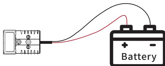
3. After selecting the appropriate charging mode, connect the charger to the battery. When the screen displays the battery voltage and input current, it indicates that charging is in progress.
