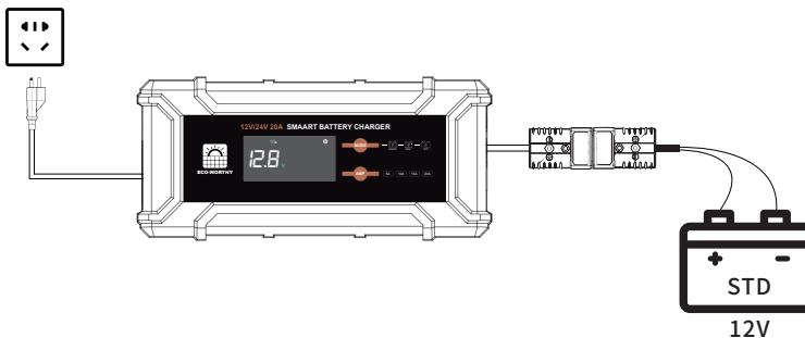
5. DC Mode: Select the DC power supply mode to connect the charger to a DC load for power supply (default is 12V 20A). Press and hold the mode button for 3 seconds to switch to 24V 10A DC. After connecting a battery, it is not possible to switch modes (the DC mode current is set to the default value and cannot be changed).
