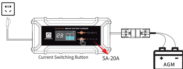
5. First, unplug the AC connector, then disconnect the Anderson connector, and finally remove the cables connected to the battery.
