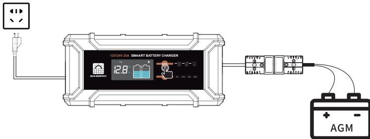
4. After connecting the charger to the battery, you can click the current switch button to adjust the current.
