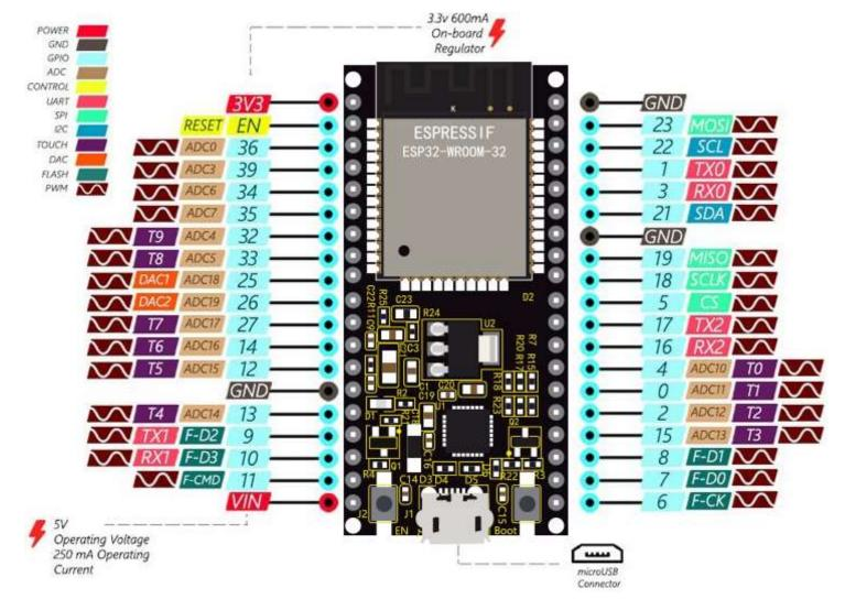
ESP32 has fewer pins than commonly used processors, but it doesn't have any problems reusing multiple functions on pins.
