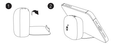
The charging case can also be used as a mobile phone holder. Unfold the phone holder as shown. Then you can place your phone on the holder.
