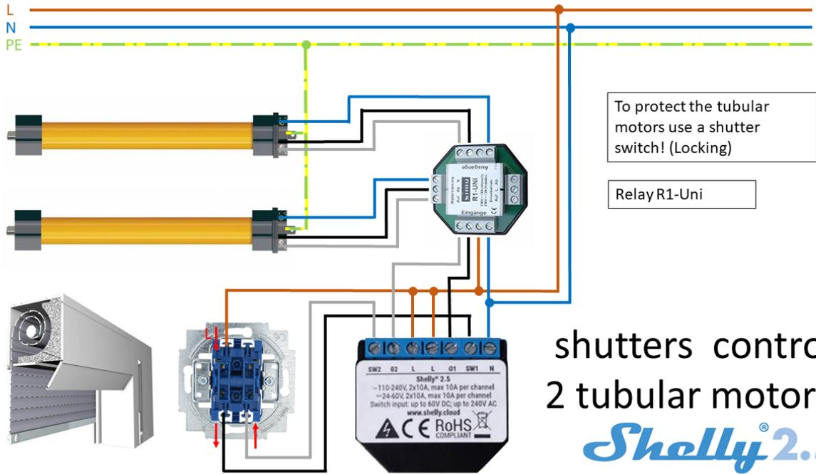
To protect the tubular motors use a shutter switch! (Locking)
