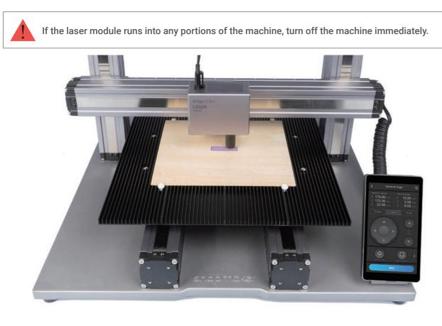
5. Tap Start, the machine will conduct an Auto Focus procedure.
