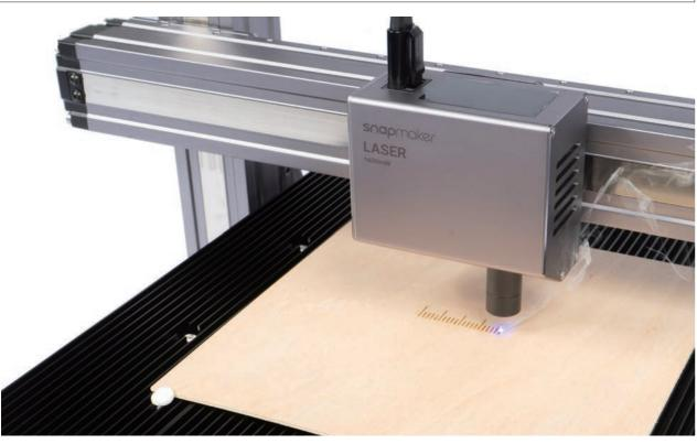
1. Remove the engraved material. Place a piece of white and blank paper (no less than 150mm x 150mm) on the center of the laser engraving/cutting platform, then fix it.
