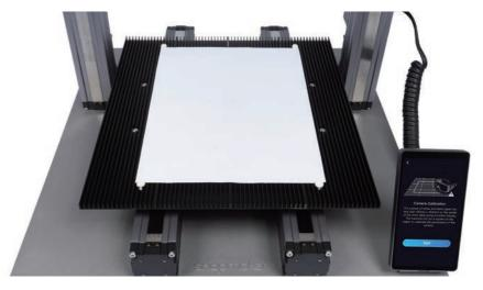
2. Tap Start, the machine will use the engraved square to calibrate the camera.
