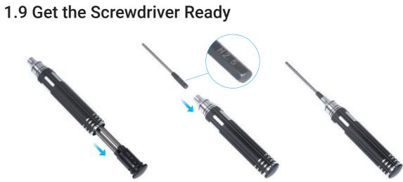
The screwdriver head H 2.5 is used for assembling the machine. The other heads are used for maintenance. Make sure the screw head holder has been put back inside of the handle before use.
