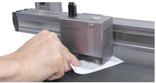
3. Keep adjusting the height of the nozzle using **Up** and **Down** buttons until there is slight resistance when you pull out the calibration card, and it should be wrinkled when you push it forward. Tap **Save** to save the calibration settings.
