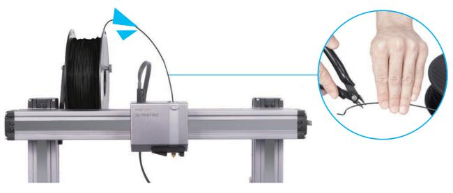
2. Tap Start on the Load Filament screen. After the temperature reaches the target temperature, tap Load and then gently push the filament into the 3D printing module until you can feel the motor pulling the filament in.
