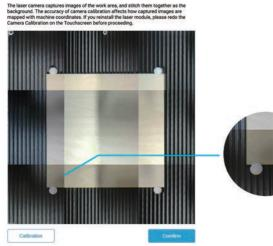
3. ① Open the test file from **Case Library** -> ② Drag the image to where the cutting will be on the captured platform -> ③ Click **Process** after configuring the settings in **Configurations** section -> ④ Use the default settings specifically configured for the test file -> (5) Generate the G-code file -> (6) Load G-code to **Workspace** -> ⑦ Set the thickness of the material -> ⑧ Click **Run** ►.
