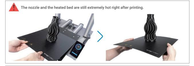
Remove the print sheet from the heated bed, place it down on a stable and flat surface. You can also use the palette knife to remove the print.
