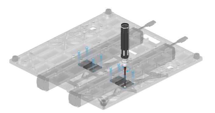
**≥ 06**/22 Attach the Z-Axis Holders to the Base Plate.
