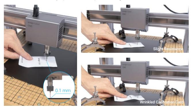
4. Tap Z+ to lift the CNC bit until it is above the clamp set, then tap Run Boundary to check if the work origin is proper. If part of the boundary runs beyond the material or the CNC bit runs into any portions of the machine, reset the work origin and run boundary again.
