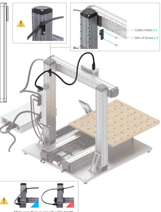
Make sure there is enough cable length for the toolhead for movement.
