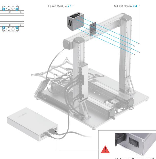
Make sure the power switch is in the Off position.
