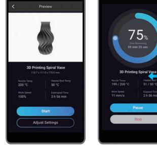
If you run into the issue of poor adhesion, swipe left on the printing progress screen and you can try adjusting the Z Offset. Or you can try leveling the heated bed again by selecting Calibration. Make sure the tip of the nozzle is clean before you calibrate the bed.
