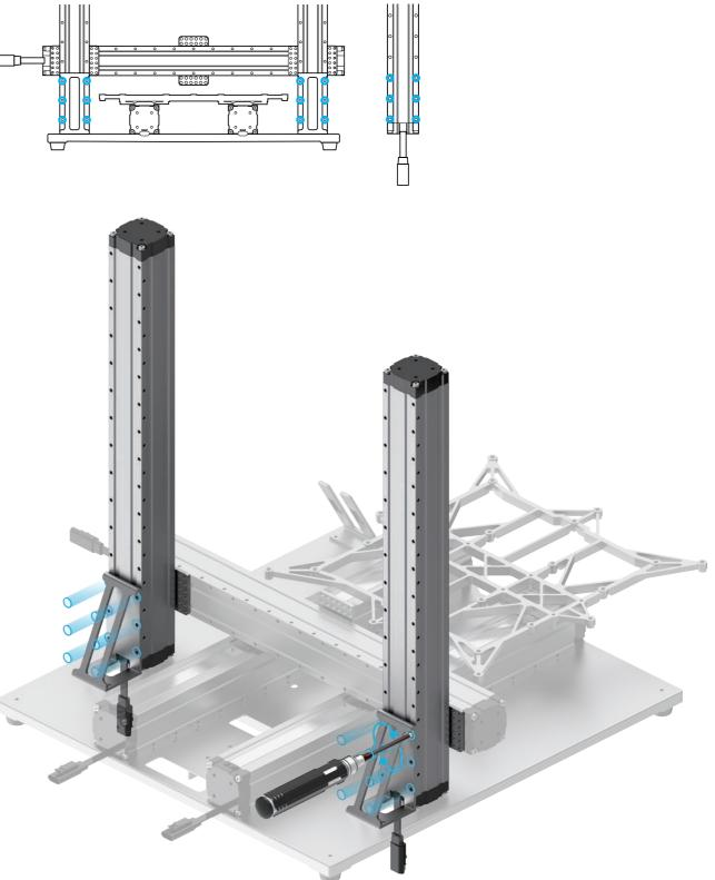
**13**/22 Tighten the screws to the bottom of the Z axes.
