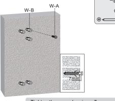
Tighten the screw leaving a 7mm space from the wall.
