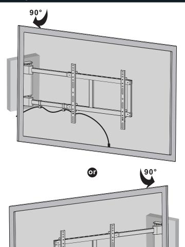
Connect the cables to your TV and route through the cable clips. **Note:** Leave slack in the cables for arm movement.
