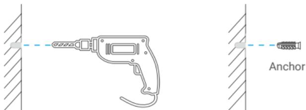
**i** It is recommended to use a drill with diameter of 6mm.
