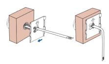
Using the steel bracket (D), make sure the up arrow is facing up and push the ribbon Cable through the slot. Then allow the screws to push through the holes so the steel bracket becomes flush with the door.
