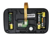
Connect the ribbon cable by pushing it onto the connection, you will feel a "Click" as it locks onto the circuit board. Make sure the cable is fitted the correct way around as shown in the image.
