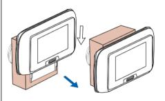
Taking extra care with the ribbon cable gently push the indoor monitor (A) back onto the steel bracket (D) and slide down to lock into position.
