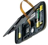
Clip the battery cover back on, the ribbon cable will fit in a small opening allowing it to come through the cover.
