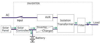
If the power from the set of photovoltaic panels is lower than the power of the connected load, the power supply will output power from the panels and the batteries, excluding charging the batteries from the panels.
