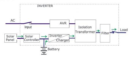
At night, after sunset, when there is a total loss of voltage from the PV panels, the load connected to the power supply will be powered exclusively by the processed voltage from the batteries.
