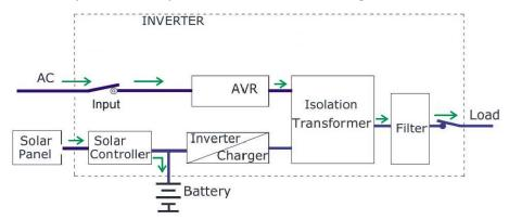
At night, after sunset, when there is a complete lack of voltage from the photovoltaic panels, the mains voltage will be transferred directly to the output of the power supply and additionally power the built-in charger that will charge the connected batteries.
