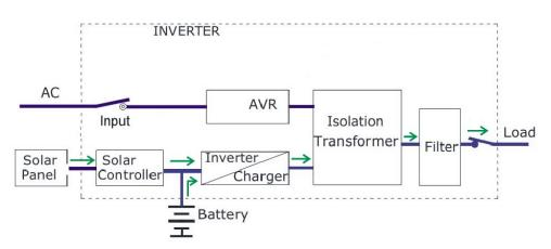
If the capacity of the connected battery pack drops below 30% of the maximum value, the voltage from the panels will not be transferred to the power supply output and will be used only for charging the batteries.
