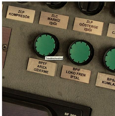
Since the locomotive will not move without rectifying the fault, this must be corrected first.
