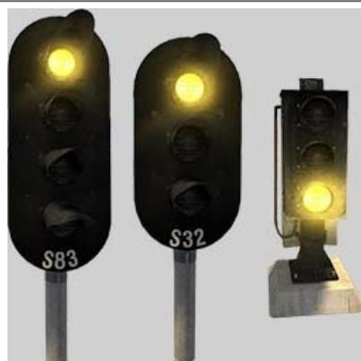
Proceed but expect to find the following signal at stop or giving access to a diverging route. The block beyond the signal is clear. The block after the following signal is either occupied, either set to a diverging route, either with no route set.
