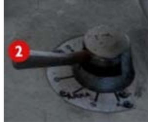
The locomotive can be moved forward with 1 step upward movement of the **Reverser**. Also it can be moved backwards with 1 step down movement of the **Reverser** too.
