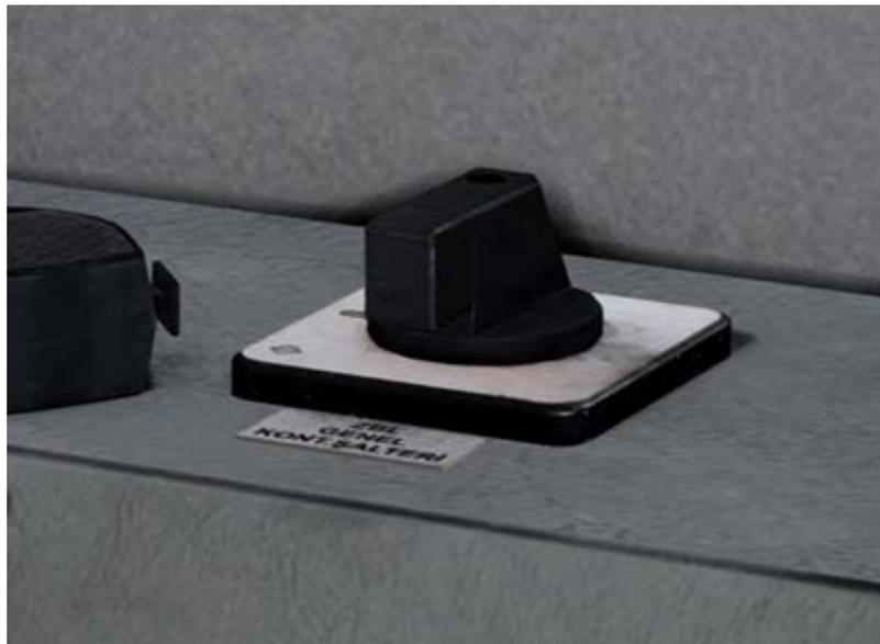
The locomotive's **Fuel Switch** must be turned on before starting (alternatively, you can press the **J** key on the keyboard). After the switch is turned on, the **Fuel Pressure** gauge slowly rises to around **2 bars**. After **2 bars** pressure is seen, the locomotive is ready to start.
