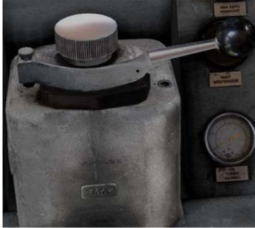
When the locomotive will be used as **Helper/Banking Engine (Ranfor)**, the train brake must also be placed in the **Ranfor (Helper)** position. For this, the small pin on the brake lever must be lifted up and the lever must be moved clockwise to bring it to the **Helper** position.
