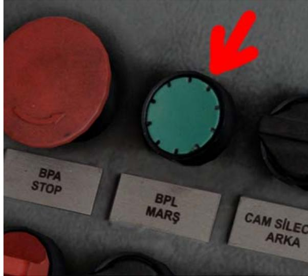
Depending on the engine temperature, the locomotive will switch from pre-lubrication to engine cranking in **30** seconds tops.
