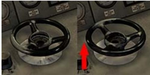
In this position, reverser is locked and cannot be moved.
