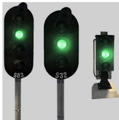
Proceed at Normal speed. Next signal is also a proceed aspect (i.e. not a stop). Two blocks beyond the signal are clear.
