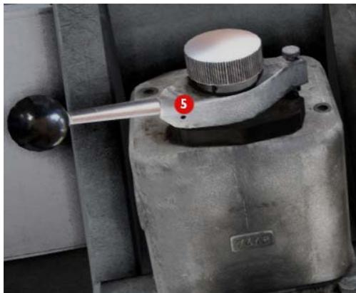
Bringing the **Train Brake** to the horizontal is the **Seri Doldurma (QckRelease)** position. In this position, the locomotive's air tanks fill faster, and the locomotive's **Brake Pipe** pressure rises up to **5.5 atm**.
