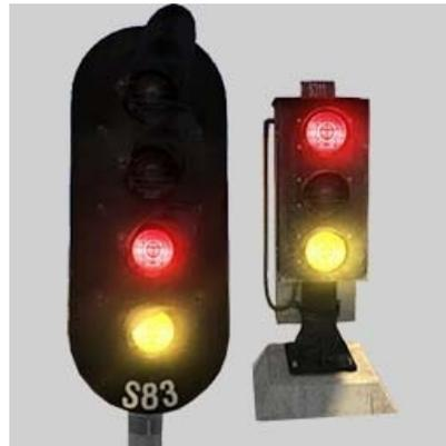
Proceed at limited speed as far as the line is clear. Be prepared to stop short of any obstruction. The signal aspect gives access to an occupied line, a non track circuited line or a non running line (e. g. turntable).
