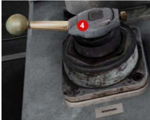
The counterclockwise movement of the **Loco Brake** lever in the cab increases the brakes, while the clockwise movement releases the locomotive brakes.
