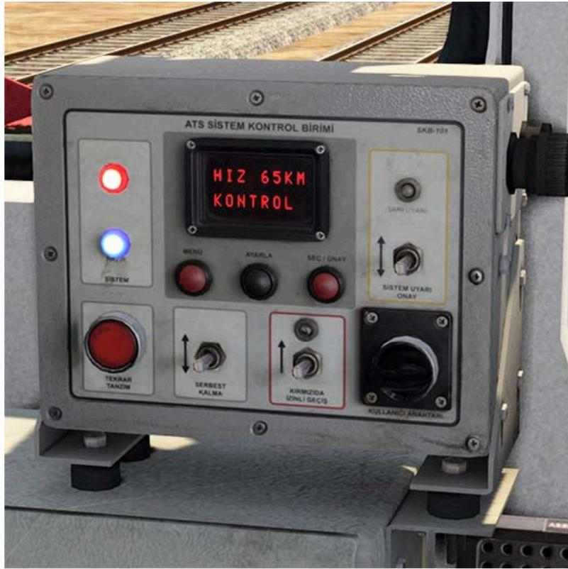
After receiving the **YELLOW WARNING**, the correct action to be taken by the engineer should be to reduce the speed of the locomotive below **65 km/h**. But in some cases, **65 km/h** speed limit control can be exited if there is too much distance to the next signal and maintenance of speed is necessary for the timetable.
