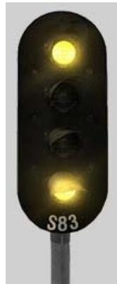
Proceed at reduced speed over points set for a diverging route. Be prepared to stop at following signal.
