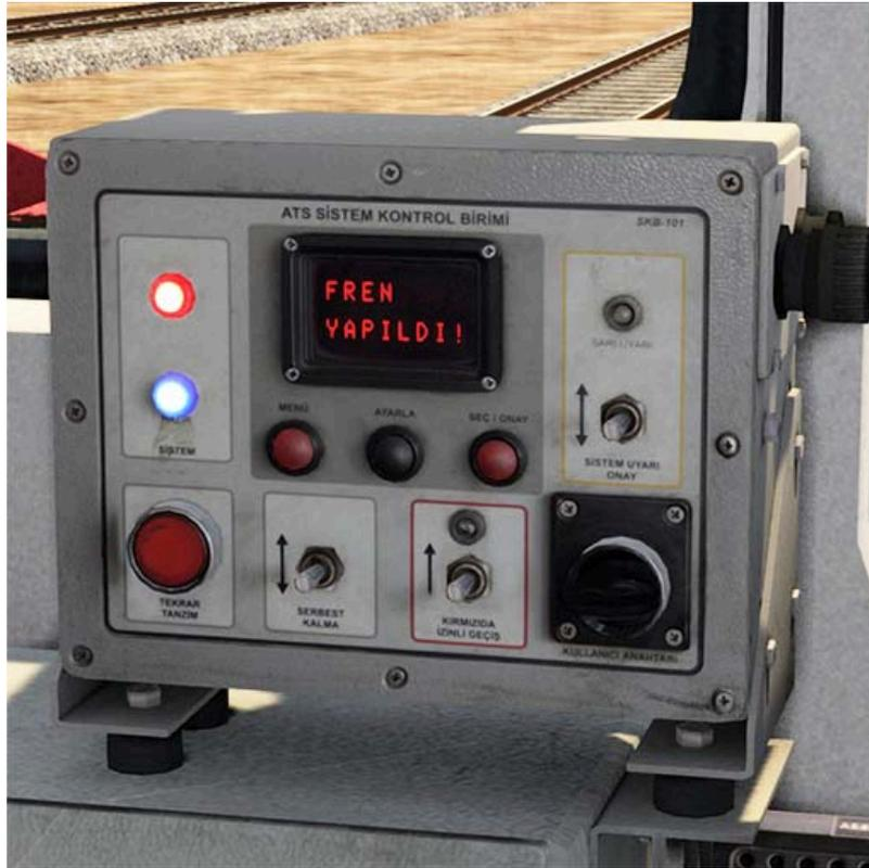
After the locomotive comes to a complete stop, the **REARRANGEMENT** button becomes active and the red light on it turns on. In addition, the text **TEKRAR TANZİM** (Rearrange) will appear on the **LCD** screen. After releasing the brakes of the locomotive, this button must be pressed before moving.
