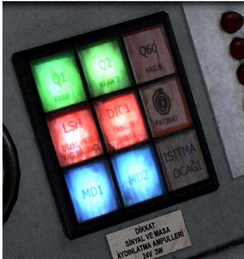
When the engine speed of the locomotive reaches **350 RPM**, **MD1** and **MD2** are disengaged and their lights go out.
