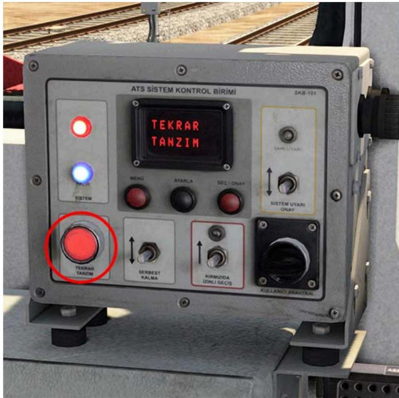
If you move without pressing this button, when the locomotive exceeds **12 km/h**, emergency braking will occur again and the above-described operations will repeat.
