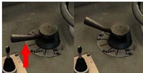
When **Valve** is in **OFF** position, if **Reverser** is moved 1 step more from forward or reverse position, it will turn into **S** position. This position stops sending current to the locomotive's traction motors but maintains the engine's **RPM**.
