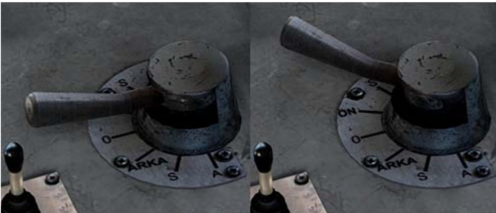
Next, the **Alternator Warning** switch needs to be turned on (alternatively, you can press the **F** key on the keyboard). If this switch is not opened, the locomotive will not move because no current will flow to the traction motors of the locomotive.
