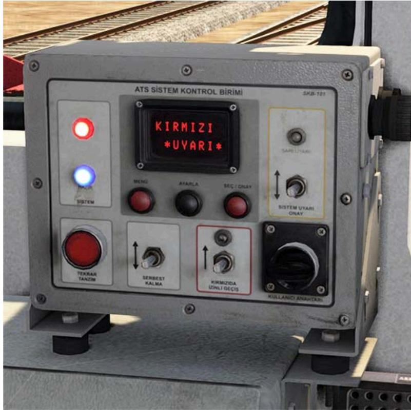
After the locomotive comes to a complete stop, the **REARRANGEMENT** button becomes active and the red light on it turns on.
