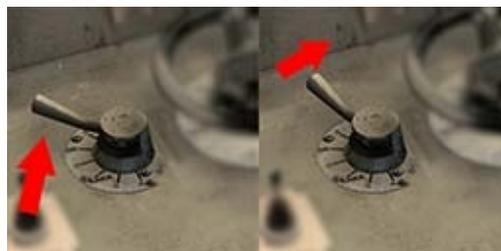
To terminate the air filling process, it is sufficient to move the **Reverser** back to the forward or reverse position or to the neutral position.
