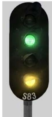
Proceed at reduced speed over points set for a diverging route. Be prepared to proceed at following signal.
