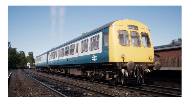
The Class 101 was one of the largest classes of first-generation Diesel Multiple Units on the British railway network. Built by Metro-Cammell Works in Birmingham from 1956, the Class 101 was made up from a number of sub-classes, making them the most numerous and possibly most successful and well known of first generation DMUs.
