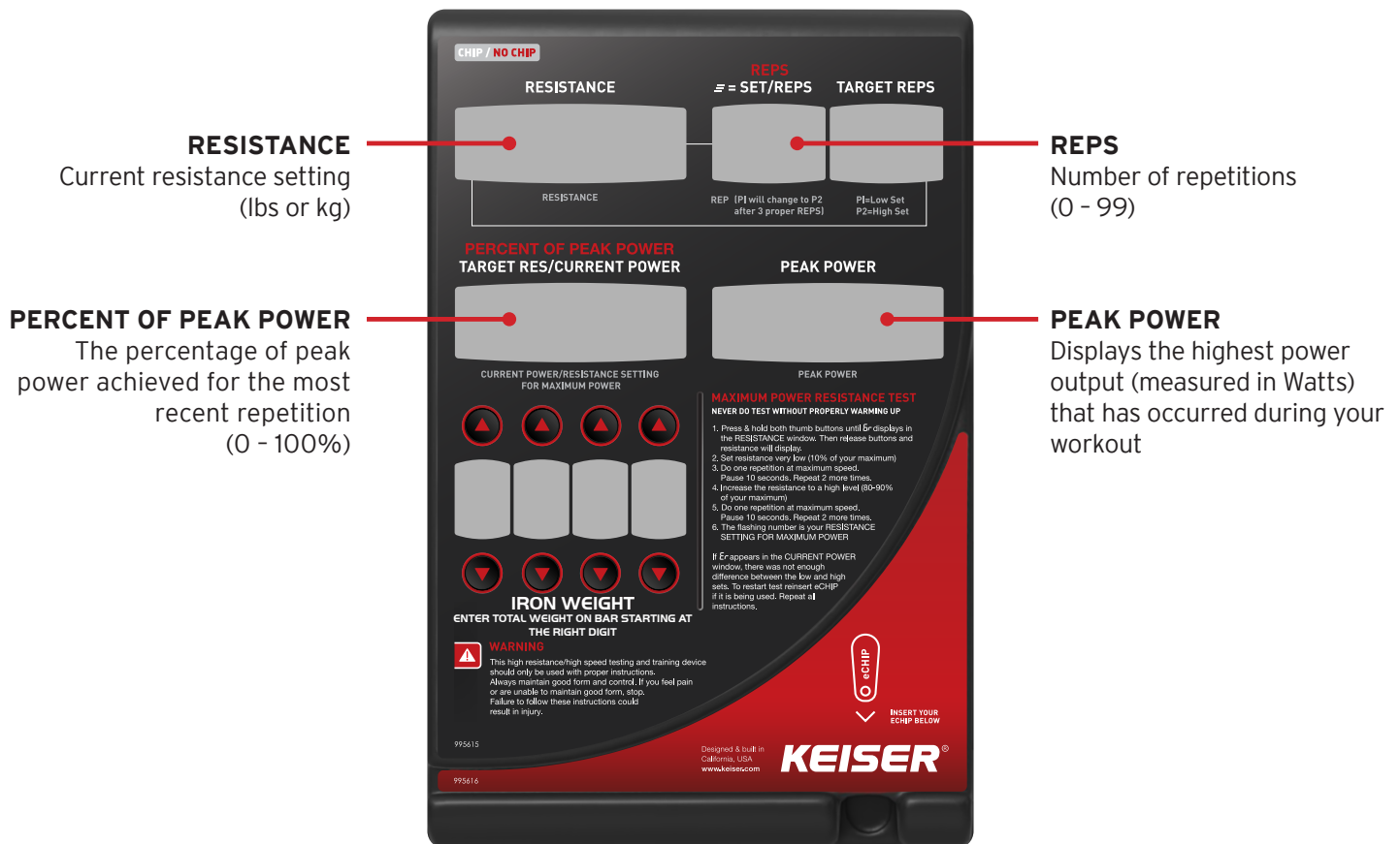
Figure 5. Power Display Overview
