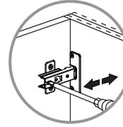
**AJUSTE DE PROFUNDIDAD / DEPTH ADJUSTMENT**
