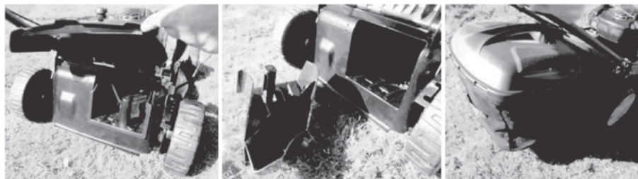
Installing the grass collector
