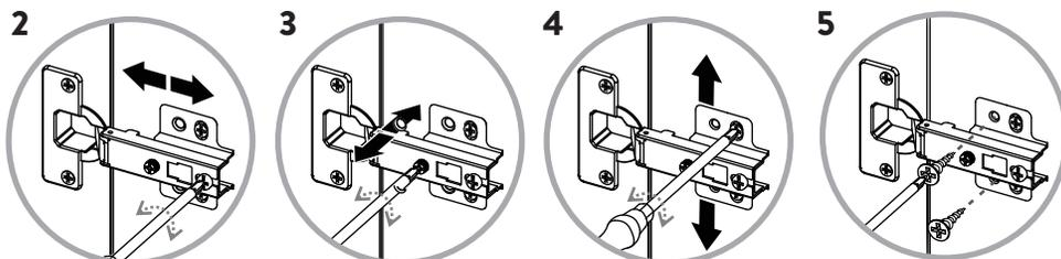
**AJUSTE DE PROFUNDIDAD / DEPTH ADJUSTMENT**
