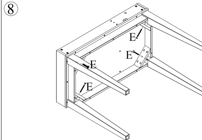
USANDO 4 PARAFUSOS E + 1 CHAVE ZETA H
