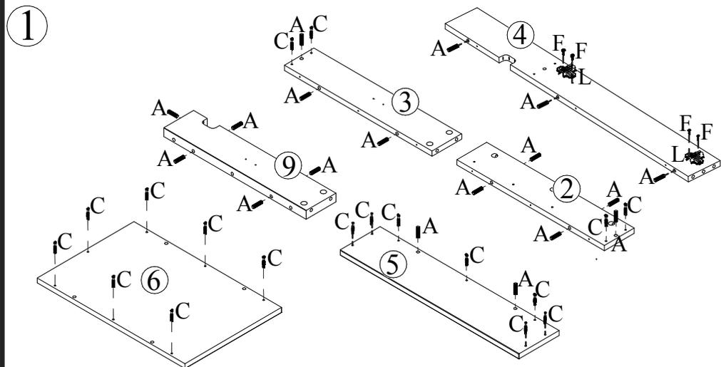
USANDO 18 CAVILHAS A + 18 PARAFUSOS C + 4 PARAFUSOS F + 2 CALÇOS PARA DOBRADIÇA L
