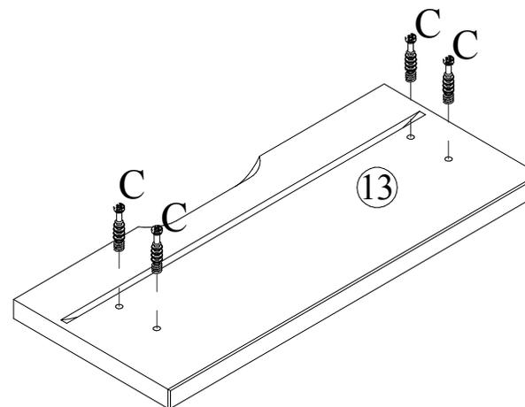
USANDO 4 PARAFUSOS C
