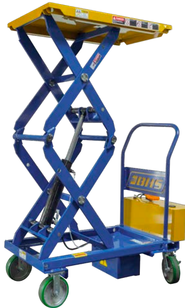
PMLTD (shown raised) features double scissors for extended range
