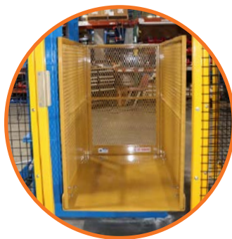
Platform carriage with caged sides ascends and descends along an upright travel track
