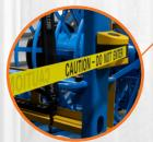
A safety yellow retractable caution tape, mounted to left and right of operator area, improves safety during cable payout.
