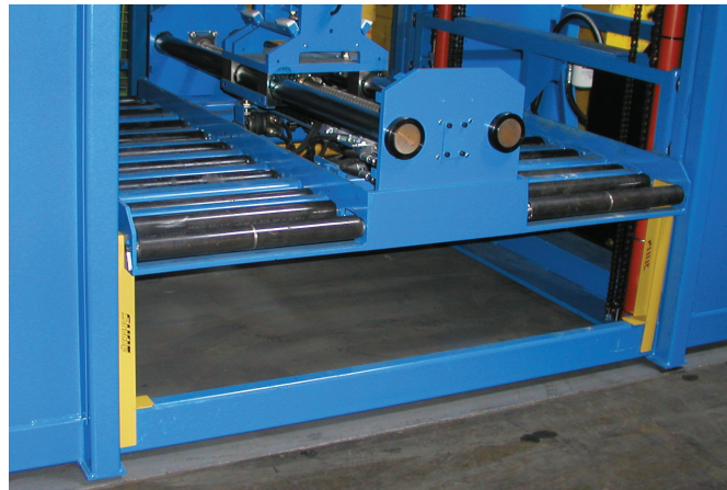
BE-TS WITH E.Q. ADJUSTMENT STOPS INSTALLED
