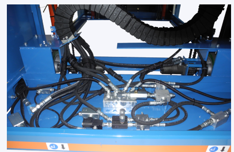
Figure 6. The BHS Battery Extractor Hydraulic System includes a simple hydraulic circuit for ease of operation, maintenance, and repairs.
