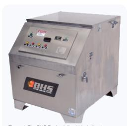
Figure 1. The BHS Recirculation / Neutralization System (RNS-4-SS pictured) controls, filters and recirculates water used for cleaning industrial batteries. The RNS-4-SS comes standard with a 200 gal (757 L) tank, a spray wand with a 10′ (3 m) hose, and a 12 V dc sump pump with float switch.
