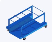
Figure 1. The BHS Cylinder Transporter (CT) provides safe and efficient handling of industrial, compressed gas cylinders by securing cylinders as the unit is transported by fork pockets or casters.
