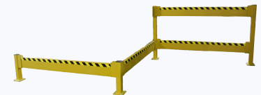
Figure 2. Structural Barrier Rail (SBR) is a heavy duty guardrail system that's designed to resist the force of a forklift strike. These all-steel barriers have an impact rating of 10,000 pounds at 4 miles per hour
