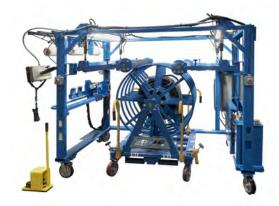
1. Operators position the SWT over the take-up drum, which sits ready on a Parallel Reel Payout or jack stand. The SWT frame is designed to roll easily into place, removing the need for additional material handling equipment for travel. Similarly, users can manually place Parallel Reel Payouts in front of master drums quickly and without ergonomic risk. Either way, users then engage the SWT's floor brake before operating the unit.
