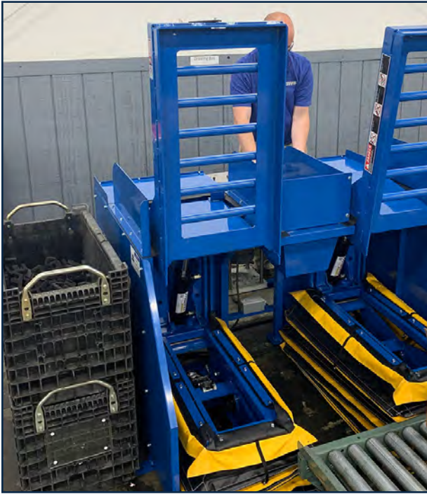
Trent Boothe tests the 90° tilt function of both Tilt Tables in tandem.
