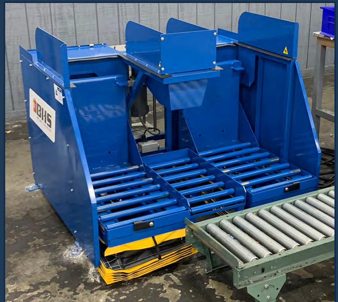
The Assembly Work Station integrates a desk with two tilt tables to keep the job’s materials close at hand. Assembled components get dropped through the middle of the table for collection and transfer down the line.
