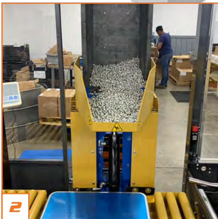
A combination Lift & Tilt Table, with a built-in chute for dispensing product, sits behind another lift table where the product is weighed.
