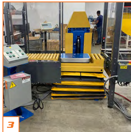
This Lift Table incorporates a scale within the tabletop for measuring the weight of the shipment.
