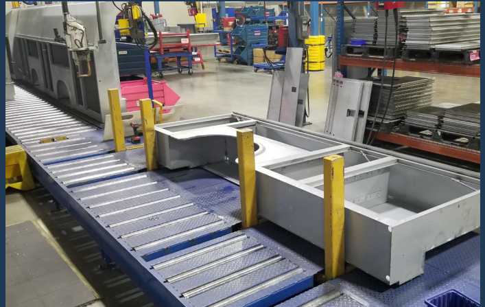
BHS' 2018 Knapheide Tilt Table handles utility truck bed compartments, tilting them 90° so workers can safely access the underside.
