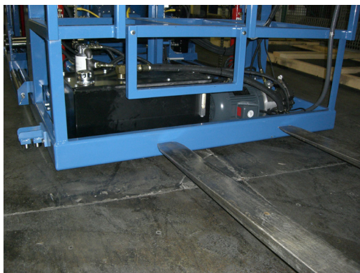
INCORRECT Pushing Extractor
