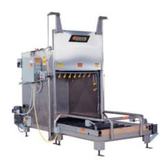
brush cleans the bottoms of the battery as it enters the wash cabinet. Often this will dislodge a fair amount of rust and debris that will collect in the BWC pan. This sand-like debris must be cleaned regularly to prevent damage to the pumps and valves.
