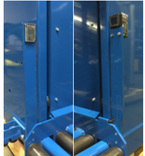
Photo-electric sensor and reflector as mounted on SL and DS extractors.
