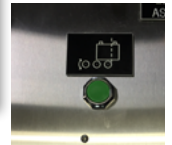
Power Roller Cutout override button mounted on dashboard.
