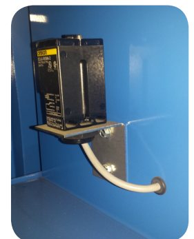
Photo-electric sensor mounted to inner frame
