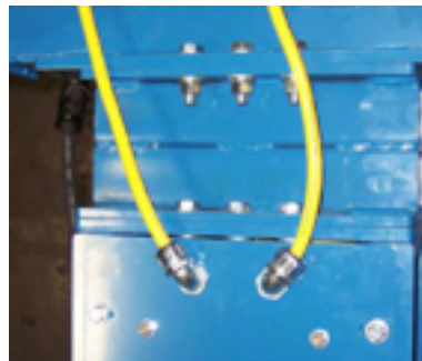
New magnet mounting utilizes independent bearing mounts for each magnet
