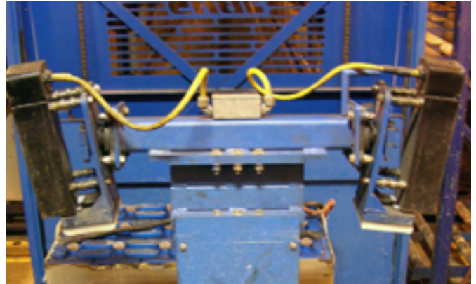
Old style magnet mount, magnets falling forward due to loose load adjusters, susceptible to damage
