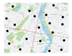
In this image, the company has used the divide and conquer heuristic to divide the 20 addresses into smaller problems of more manageable size. The company can then brute-force these individual sections and put them back together. However, with a larger problem, brute-forcing could again run into time issues. In that case, the company could use other heuristics to find an efficient solution for each small sub-problem.
