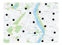
For example, a company needs to deliver to the 20 addresses shown on this map. If it were to brute-force this problem, approximately  $2.4 \times 10^{18}$  obtained solutions would need to be calculated. This would take an impractical amount of time, and so the company needs to use a better way to find a solution.
