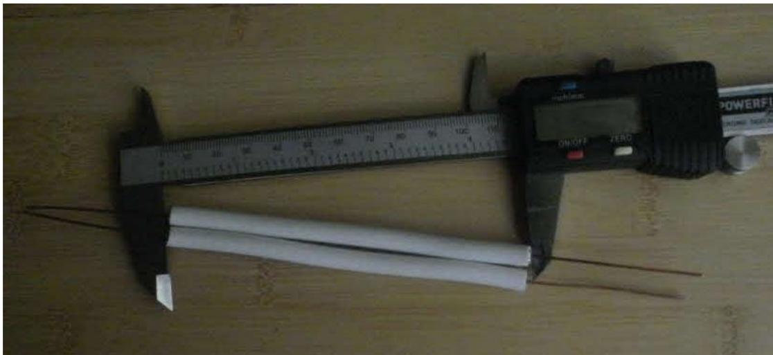
When assembling the components, use a small piece of electrical tape between each element to prevent short circuits. Carefully push each tail between the outer insulation and the braid. Use electrical tape or heat shrink tubing to seal the joins.
