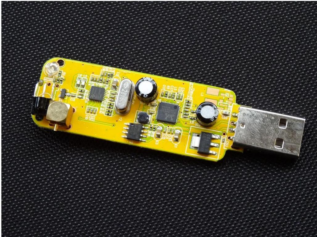
Figure 3 - The inside detail of a USB SDR
