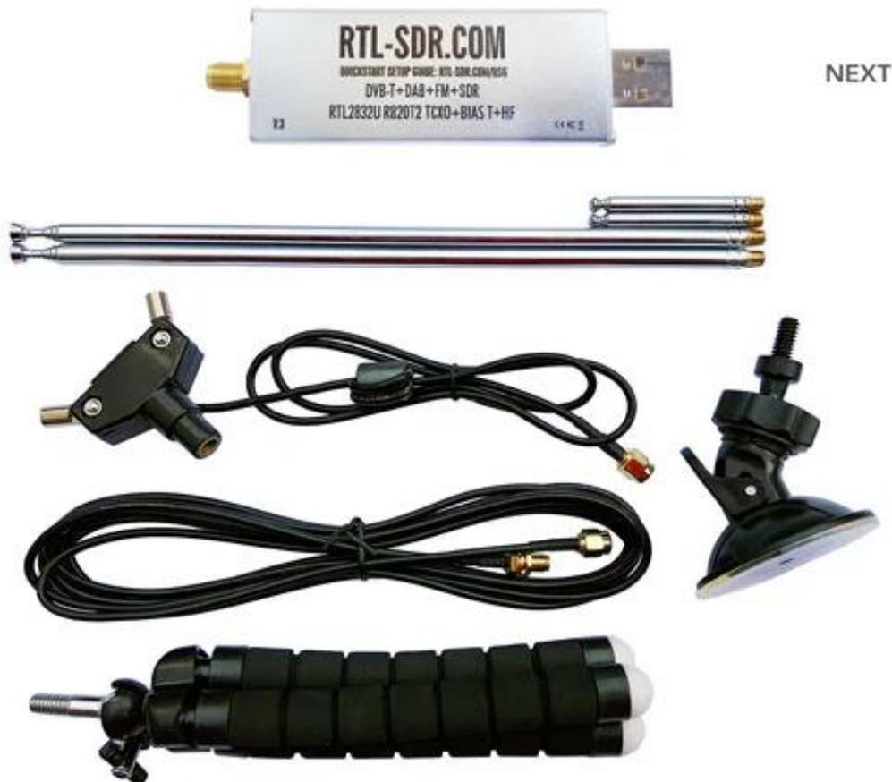
This kit uses an [SMA](#) antenna connector. These are more common, and are often used for Wi-Fi routers. If you are going to use anything other than the included antenna, then you will need to buy, or build, an adapter such as the SMA (Female) to BNC adapter shown below.
