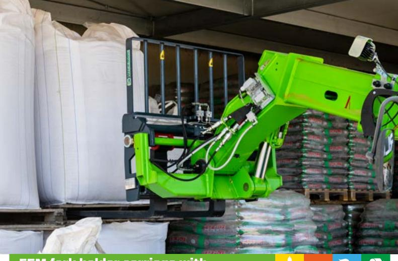
FEM fork holder carriage with positioner - hydraulic side-shift
