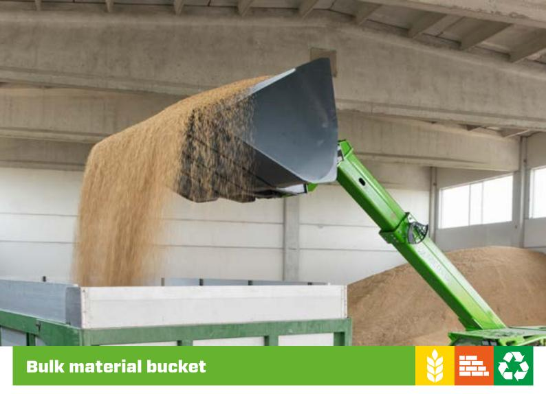
Bucket designed for handling bulk material having a maximum density of 900 kg/m³
