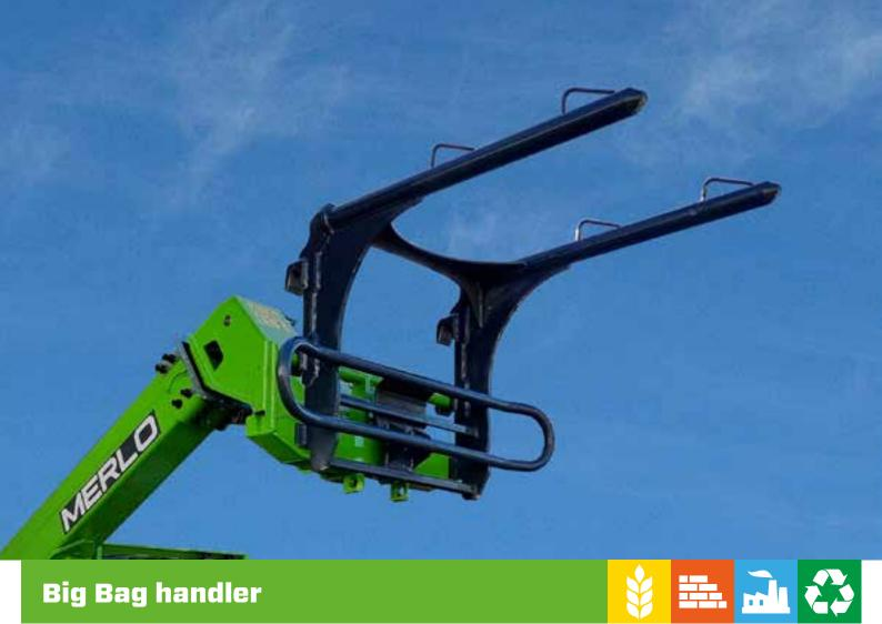
Attachment designed to lift and handle big bags using 1, 2 or 4 hooks
