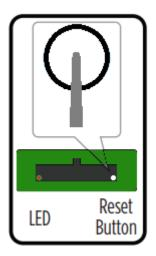
If the interface fails to function, press and release the reset button, then repeat the programming process from step 3 to try again.
