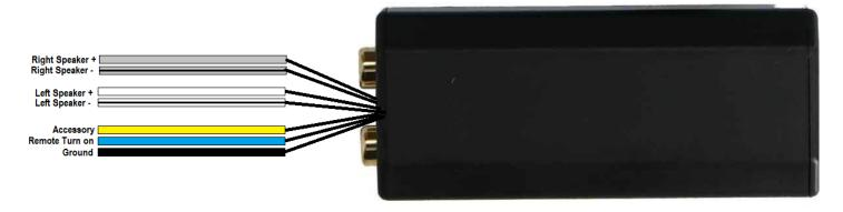
Installation: The WM-LOCKN should be installed on a stereo's speaker output wires or the output wires on an OEM amplifier of up to 30 watts per channel. These wires can be found behind the stereo in the dash, on the outside of an OEM amplifier, or on the input terminals on the OEM speakers.
